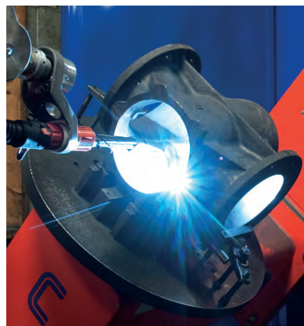
Figure 3. Robotic welding of nickel seat
